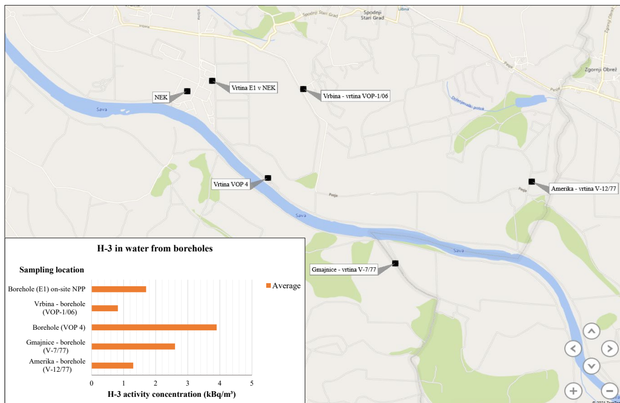
Figure I6: Review of monthly averages of activity concentrations of H-3 in water from the boreholes. The water from the boreholes is not used as drinking water or process water, but only for tracking liquid discharges from the Krško NPP.
