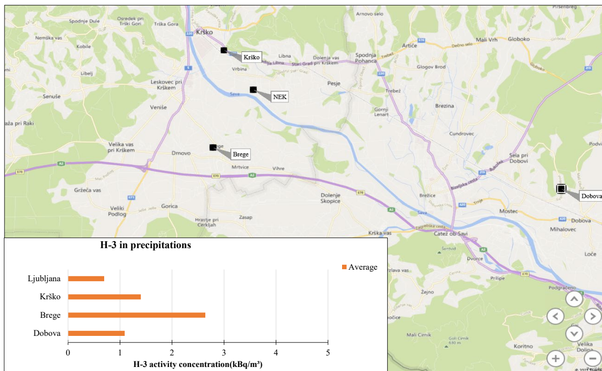
Figure I7: Review of monthly averages of activity concentrations of H-3 in precipitation at sampling locations in the vicinity of the Krško NPP. The activity concentration of H-3 obtained at the reference location (Ljubljana) is compared with values in the vicinity of the Krško NPP.
