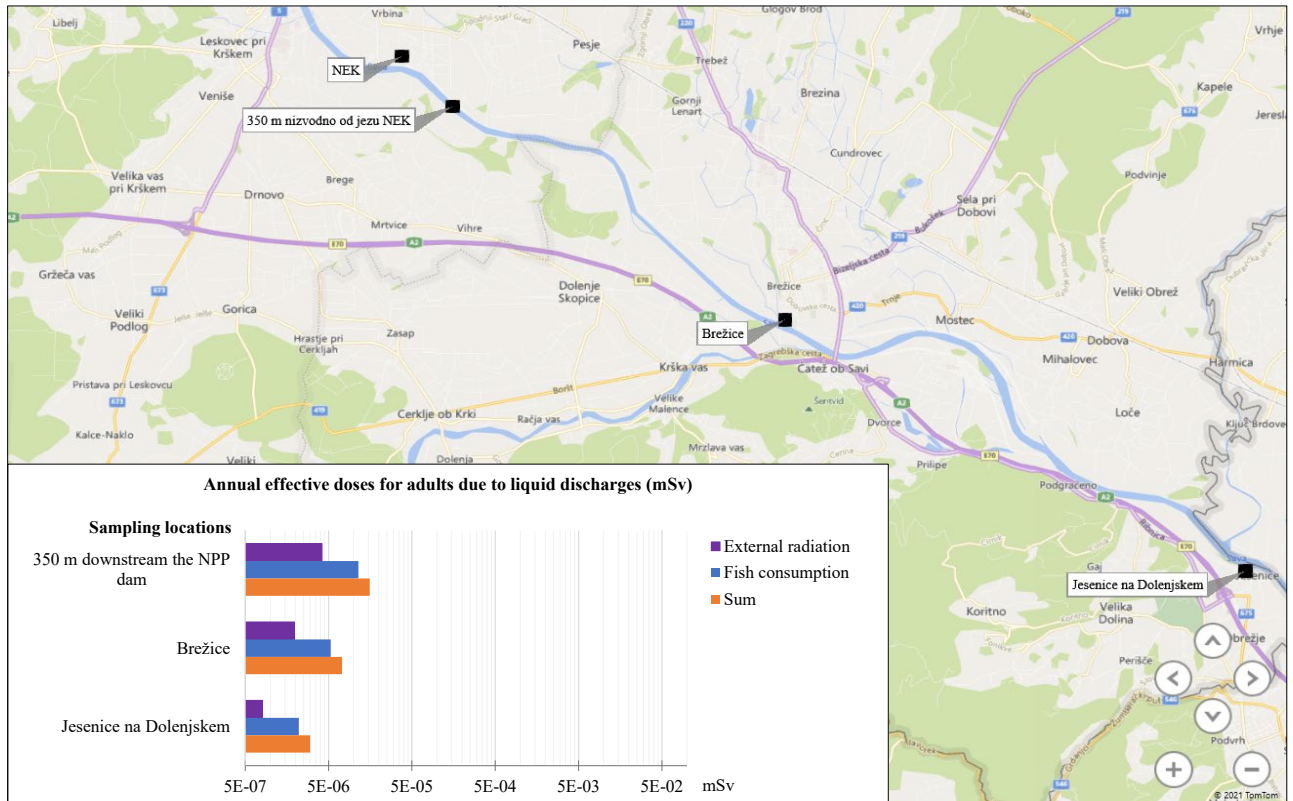
Figure P2: Review of estimated annual effective doses for artificial radionuclides for liquid discharges from the Krško NPP in 2021. The scale is logarithmic.
