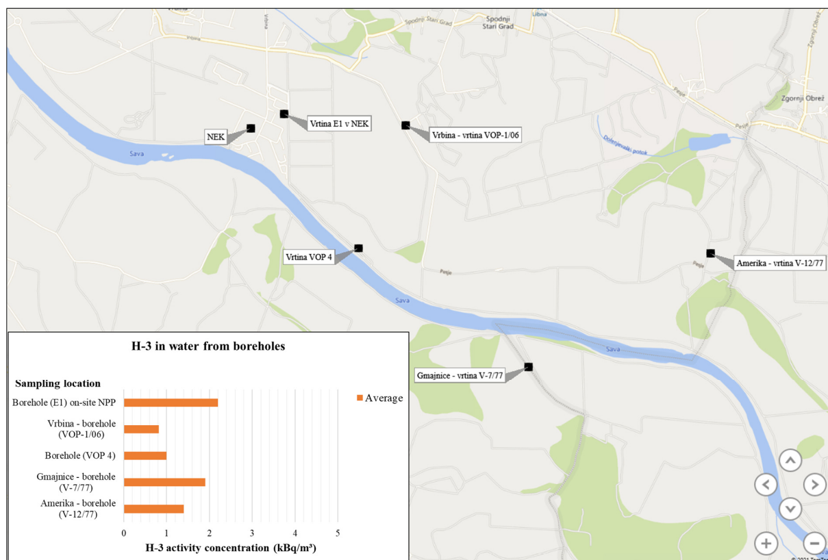
Figure I6: Review of monthly averages of activity concentrations of H-3 in water from the boreholes. The water from the boreholes is not used as drinking water or process water, but is only used for tracking liquid discharges from the Krško NPP.
